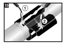
Remove the remaining sleeve release liner and wrap the sleeve loosely around the pipe, ensuring the appropriate overlap. Before finishing wrapping the sleeving side of the underlap until the backing starts to recover. Then use a roller to secure the underlap to the pipe. 2. gently heat the adhesive side of the closure seal until it appears glossy.
