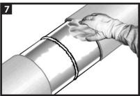
Using a dry, grease and lint-free cloth, wipe clean or air blast the steel and coated areas to remove foreign materials. If necessary, provide additional heat to ensure the surface temperature is 30-50°C (86-120°F).
