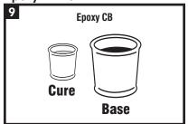
Follow the Preparation, Mixing and Application instructions provided with the supplied Canusa Epoxy. For bulk quantities: mix the primer cure with the primer base (4 parts base to 1 part cure by volume). Sitr for a minimum of 30 seconds to assure uniform
