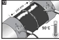
Heat the conductive bands with the propane torches until underlying mainline coating reaches a temperature of at least  $90^\circ\text{C}$ . Use the sliding door to check temperature of mainline coating. Remove the conductive bands when finished.
