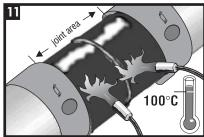
Pre-heat the epoxy to a temperature of 100°C (194°F) with at least 2 propane torches or an induction heating coil. Use a contact pyrometer to verify the correct temperature has been reached. The conductive bands should stop direct flame from hitting mainline coating. If a film does develop on the mainline coating use a surface abrasion tool to remove it.
