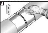
Ensure that the mainline coating edges are beveled to 30° minimum. If there is the presence of oil, grease, or other surface contaminants; clean the exposed steel and adjacent pipe coating with an approved solvent cleanser.
