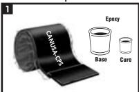
GTS-PP-120 3L sleeves are shipped pre-cut with a pre-attached closure. The sleeve adhesive is protected from contamination by an inner liner. The joint completion system includes an epoxy primer.
