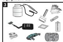
Propane tank, hose, torch & regulator Power grinder with grind wheel of a Grade 40 grit rating Canusa conductive bands Digital thermometer with suitable probe Knife, J roller, rags & approved solvent cleanser Epoxy applicator pad, wet film thickness gauge Standard safety equipment; gloves, goggles, hard hat, etc.
