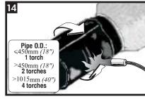
Using an appropriate propane torch, begin at the centre of the sleeve and heat circumferentially around the pipe, using broad strokes. If utilizing two torches, operators should work on opposite sides of the pipe.
