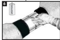
Ensure that the mainline coating edges are beveled to 30°. Clean exposed steel and adjacent pipe coating with a solvent cleanser to remove the presence of oil, grease, and other contaminants. Cleansing of coating overlap not required for AE coating type.
