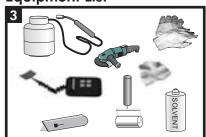
Propane tank, hose, torch & regulator Appropriate tools for surface abrasion Knife, noller, rags & approved solvent cleanser Digital thermometer with suitable probe Standard safety equipment; gloves, goggles, hard hat, etc.
