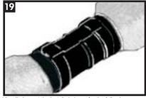
Visually inspect the installed sleeve for the following: Sleeve is in full contact with the steel joint.
