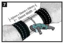
Ensure that the pipe is dry and surface moisture has been removed prior to surface preparation. If required, use propane torch heating to raise the steel temperature accordingly (to > 40 deg C). Prepare the bare steel cutback to ISO 8501:1 class St 3 preparation standards using mechanical wire brush or grinder equipment.
